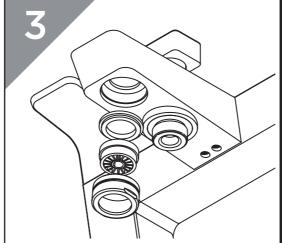
Replace the aerator, ensuring the washer has been fitted. Secure in place by tightening with suitable spanner.
